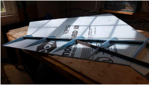
Blue Wing #3 (6 foot wingspan) - internal layout
